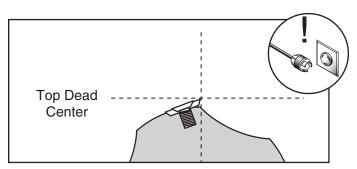
Figure 12. Cutterhead insert at top-dead-center.
